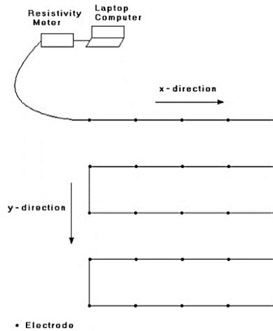
Figure 1 Preparation of grid electrodes for 3-dimensional survey[11].
